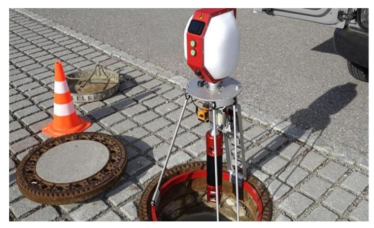
Envirosight Quickview 360 Maintenance Hole Scanning Pole Camera system
